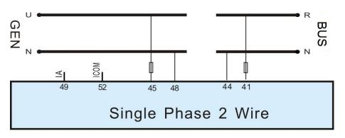
Fig. 7 Single Phase 2 Wire Application Diagram
