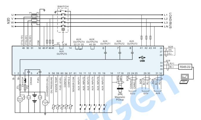
Fig. 4 HGM9510 Typical Application Diagram
