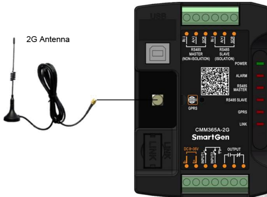
Fig.2 – GPRS Antenna Connection Schematic Diagram
