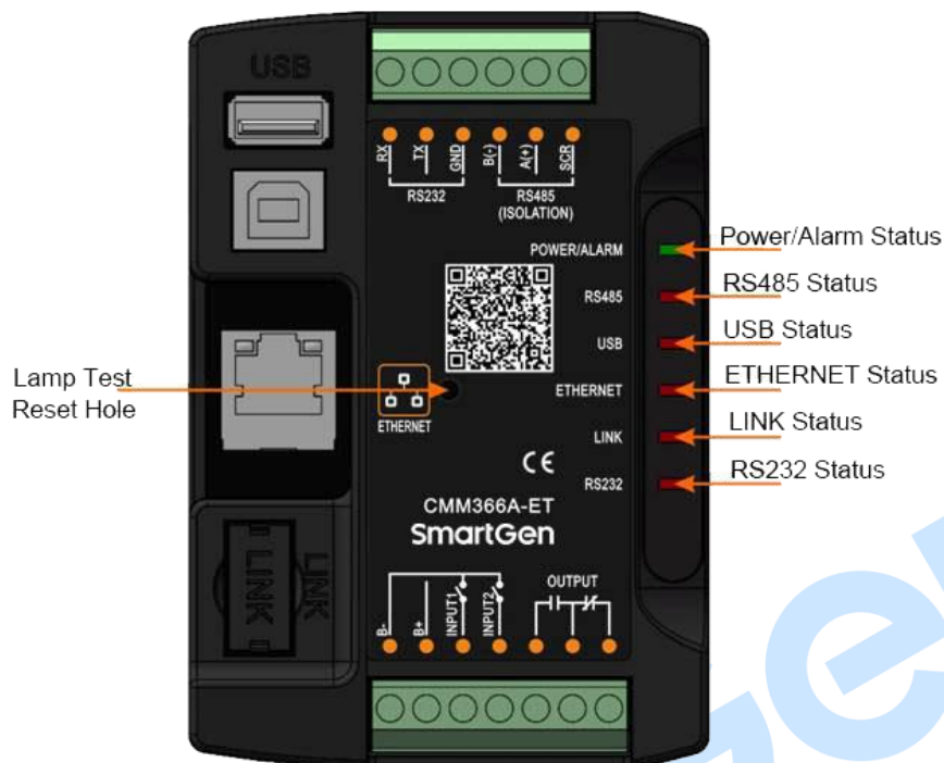
Fig.1 – CMM366A-ET Front Panel Diagram
