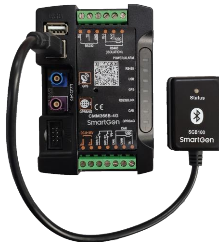
Fig.9 – USB and SGB100 Module Connection Diagram
