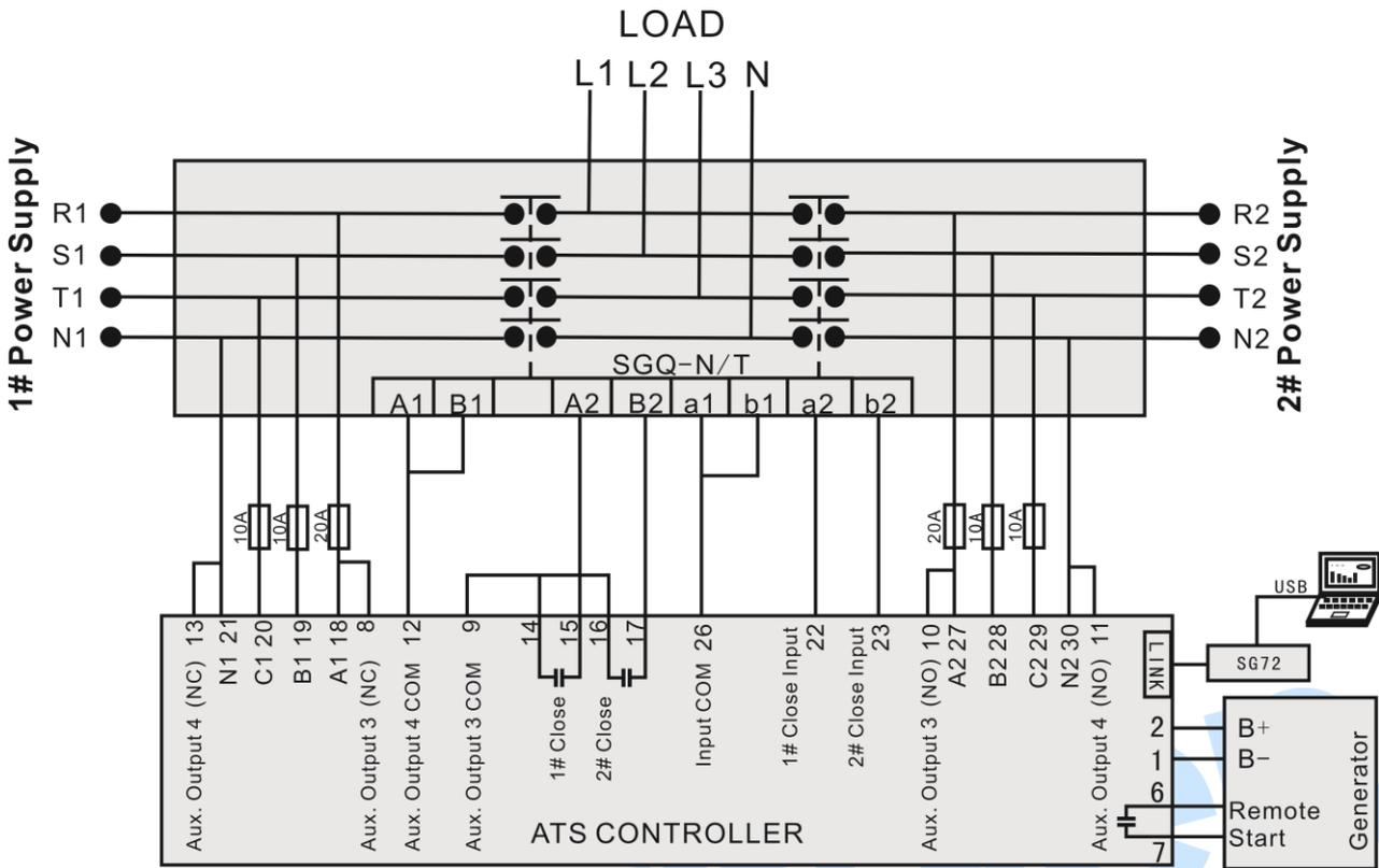
Fig. 3 SGQ-N/T Wiring Diagram
