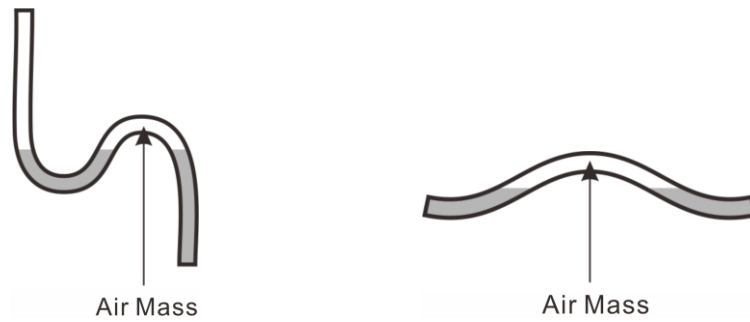
Fig. 3 – Incorrect Pipe Connection Methods
